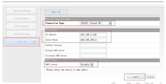
Tips: Users can configure VAP11N to connect to wifi hot spot, then revise VAP11N IP manually, and close the DHCP service, finally turn off and reboot VAP11N.
